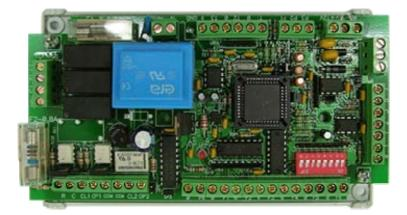
Main Controller All-IN-ONE<sup>™</sup> Fan-Coils with proportional outputs (3-wire) for Cool and Heat valves, with Native BACnet Protocol
