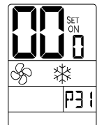
Fan ON delay in cooling (seconds)
