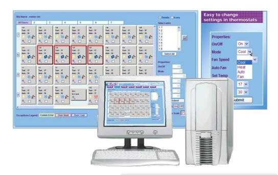
Web based, mini BMS software, for controlling small to medium sized HVAC networks
