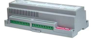
The CTU adaptability is an ideal solution for OEM's and Contractors who require "tailor made" controller configured according to their particular requirements at a The CTU controller offers advanced communication protocol capabilities, such as Modbus or BACnet for B.M.S control and selectable power supplies 24VAC, 110VAC or 230VAC.
